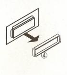
2. Insert the keys supplied with the unit at both sides of the unit as shown in figure until they click. Pulling the keys makes it possible to remove the unit from the dashboard.
