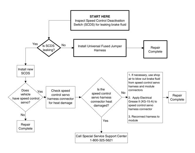
Flow Chart #2 shows the repair procedure for 1999 through 2003 Windstar vehicles.
