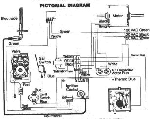
SKPORTANT If any original wire has to be replaced, it must bereplaced with the type 105 C or its equivilant.
