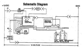
\*CB = Circuit Breaker on/off HV = High Voltage
