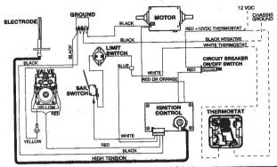
MPORTANT: If any original wire has to be replaced, it must be replaced with type 105°C or its equivalent. Terminal Block on 85 Models only.
