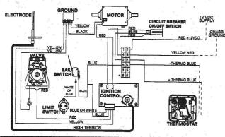
IMPORTANT: If any original wire has to be replaced, it must be replaced with type 105°C or its equivalent. "Terminal Block on 85 Models only.
